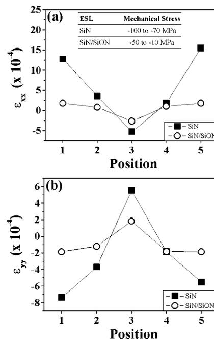
**Figure 2.** (a) Longitudinal lattice strain  $\epsilon_{xx}$ , and (b) transverse lattice strain  $\epsilon_{yy}$  for  $\text{Si}_3\text{N}_4$  and  $\text{Si}_3\text{N}_4/\text{SiO}_x\text{N}_y$  ESL samples measured from CBED patterns taken from the Si substrate at the positions indicated by the numbers 1 to 5 on Fig. 1a. Inset in (a) shows the blanket film stress measurement for  $\text{Si}_3\text{N}_4$  and  $\text{Si}_3\text{N}_4/\text{SiO}_x\text{N}_y$  films.
