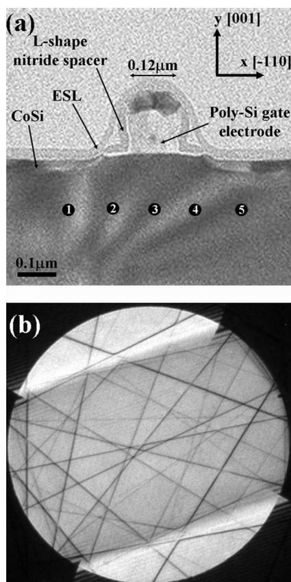
**Figure 1.** (a) Cross-sectional bright-field TEM image of an n-channel MOSFET with the CBED measurement positions indicated by the numbers 1 to 5. (b) An example of one of the CBED patterns obtained from the sample shown in (a) with the electron beam aligned along the (230) zone axis.
