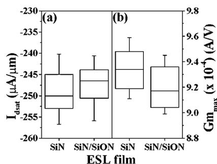
**Figure 4.** Comparison of (a) saturation drain current ( $I_{dsat}$ ) and (b) maximum transconductance ( $G_{m,max}$ ) between  $Si_3N_4$  and  $Si_3N_4/SiO_xN_y$  ESL samples, for p-channel MOSFETs, in the form of a box plot. The ESL shows no appreciable effect on the electrical behavior.
