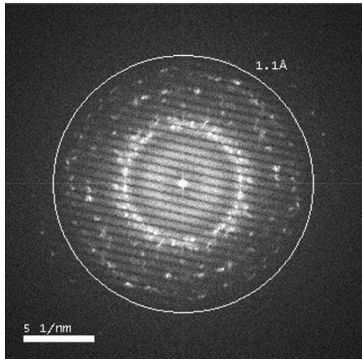
**Figure 1.** Youngs fringe experiment showing the resolution of the environmental Titan under 0.5mbar  $N_2$  pressure. The fringes are easily recognized up to  $9.2 \text{ nm}^{-1}$  corresponding to  $1.1 \text{ \AA}$ .
