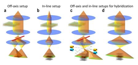
Figure 1 | Schematic view of microscope setups: (a) off-axis and (b) in-line electron holography.(c) Shows how the in-line data can be acquired immediately after switching off the biprism, in a fully automated fashion by simply shifting the image. (d) Shows how the data have been acquired for the present work: the biprism was retracted, and the sample was slightly shifted to allow investigation of identical specimen areas by both methods.
