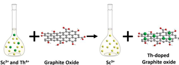
Figure 1 The preferential sorption of \text{Th}^{4+} on graphene oxide surface.
