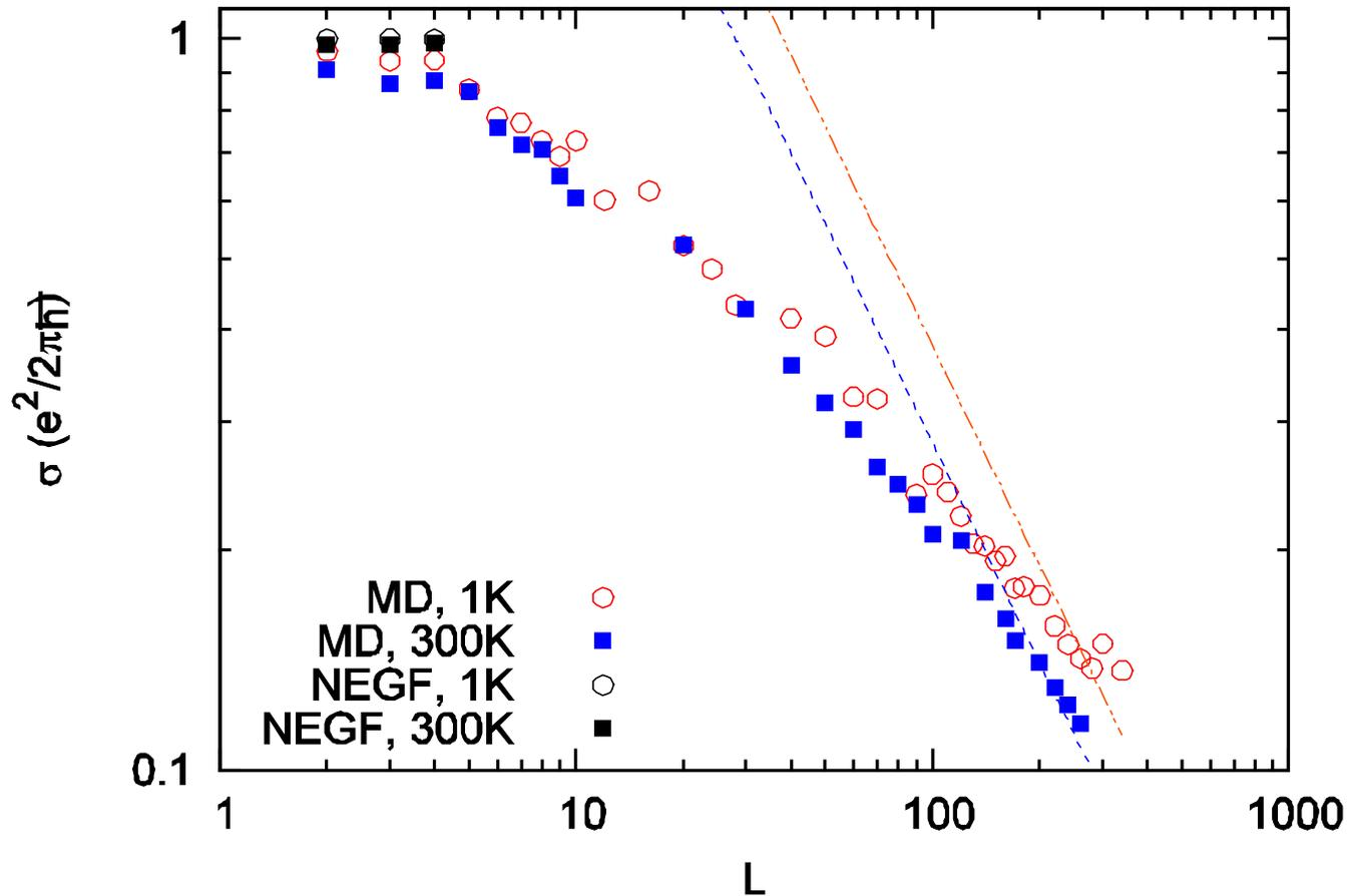
Electronic conductance vs center junction size  $L$ . Electron-phonon interaction strength is  $m=0.1$  eV. From Lü & JSW, arXiv:0803.0368.
