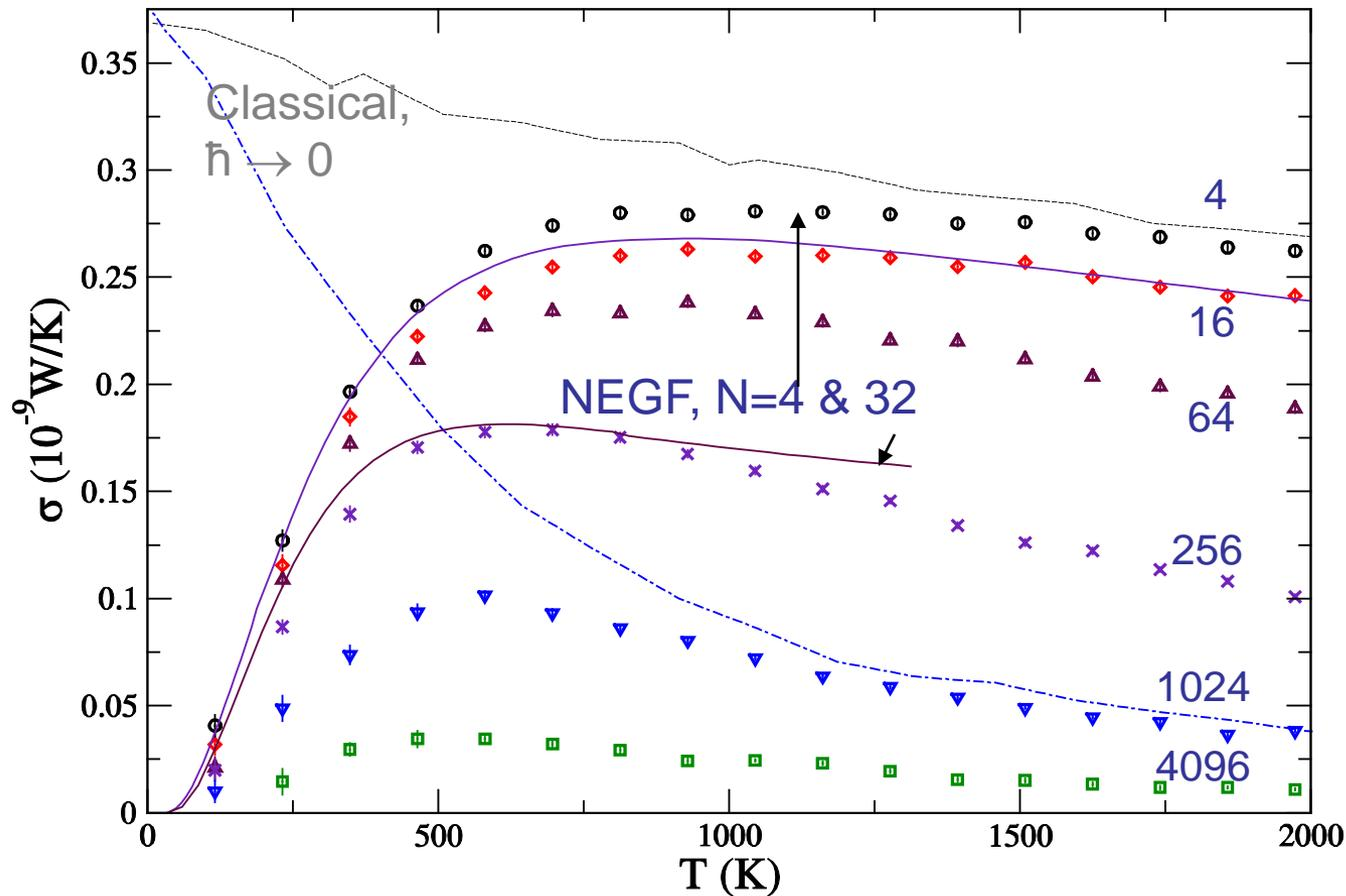
1D chain with quartic onsite nonlinearity ( $\Phi^4$  model). The numbers indicate the length of the chains. From JSW, PRL 99, 160601 (2007).
