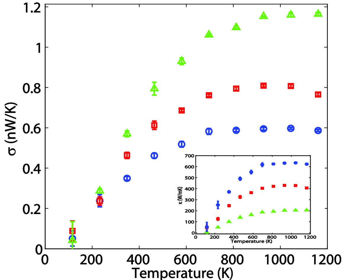
Temperature dependence of the thermal conductance (and conductivity) for lengths 4.26 (green), 12.8 (red) and 25.6 (blue) nm, respectively. JSW, Ni and Jiang, PRB 2009.
