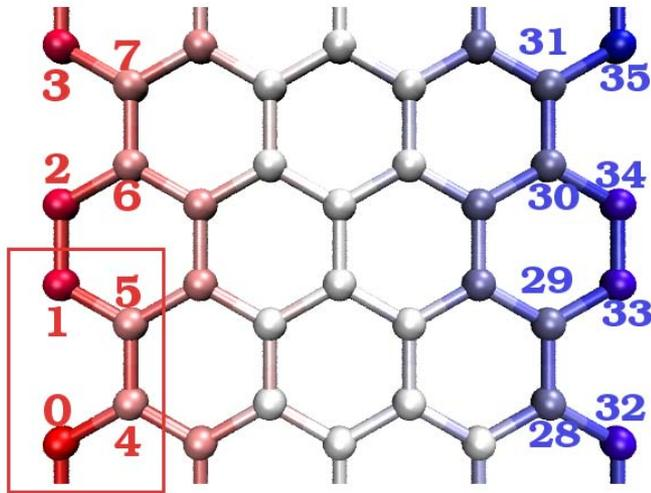
Sites 0 to 7 are fixed left lead and sites 28 to 35 are fixed right lead. Heat bath is applied to sites 8 to 15 at temperature  $T_L$  and site 20 to 27 at  $T_R$ . JSW, Ni, & Jiang, PRB 2009.
