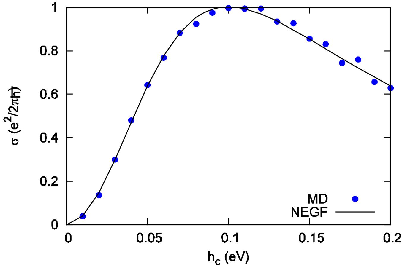
Nearest neighbor hopping model with two sites in the center, lead hopping  $-h_l = 0.1$  eV, varying the center part hopping term. From Lü & JSW, arXiv:0803.0368. For NEGF method of electron-phonon interaction, see Lü & JSW, PRB 76, 165418 (2007).
