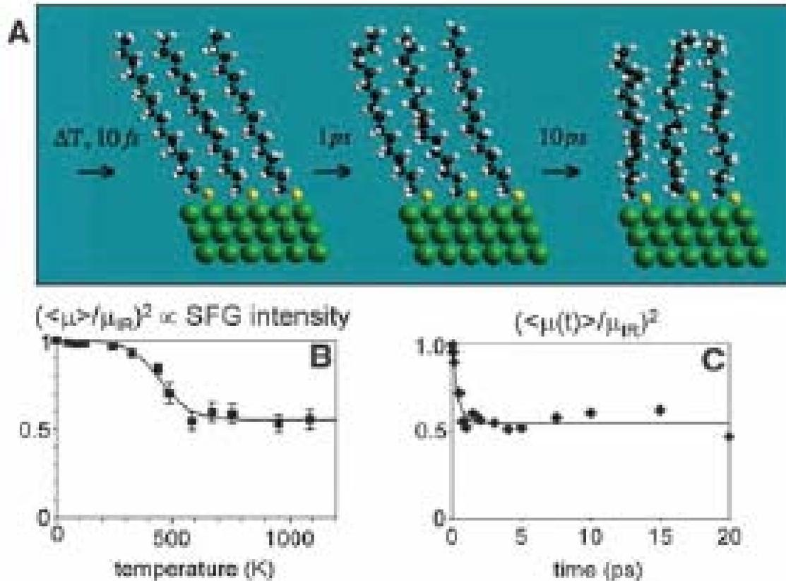
The experimentally measured thermal conductance is 50pW/K for alkane chains at 1000K. From Z Wang et al, Science 317, 787 (2007).
