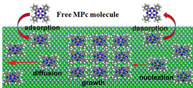
**Figure 1.** Schematic drawing of processes relevant in organic thin-film growth on metal surface, such as adsorption, desorption, diffusion, nucleation and growth of islands. The MPc molecular structure is also shown.
