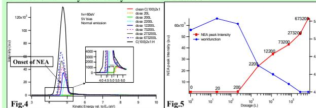
The results clearly show that the surface remained PEA below 200L dosage and then changed to NEA with the NEA peak intensity increasing logarithmically with 1,3-butadiene coverage (Fig. 5). At the same time the lowering of vacuum level indicates that the work function was also decreased accordingly (Blue line in Fig. 5).
