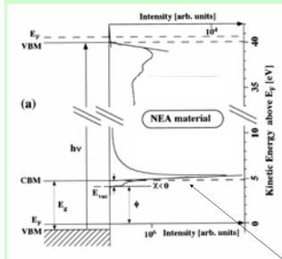
**Fig. 1** NEA means the conduction band minimum (CBM) of certain material lies above the vacuum level. So the electrons excited into the conduction band can be thermalized to the CBM and emitted into vacuum without any energy barrier which leads to a very sharp peak at the low electron kinetic energy part in UPS.
