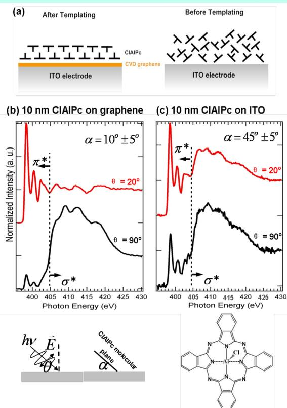
(a) Schematic of the proposed molecular packing structure for CIAIPc molecules before and after templated by CVD graphene. Angular-dependent N K-edge NEXAFS spectra for 10 nm CIAIPc film on (b) CVD graphene modified ITO and (c) bare ITO electrodes. The molecular structure of CIAIPc is shown at the bottom of the Figure.
