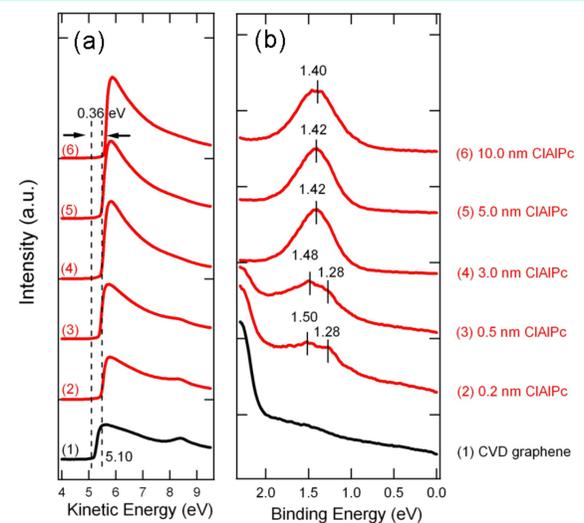
UPS spectra of CIAIPc on CVD graphene (a) at the low kinetic energy region and (b) at the low-binding energy part near the  $E_F$  region.
