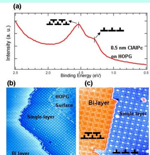
(a) UPS spectrum near the  $E_F$  region for 0.5 nm CIAIPc on HOPG surface (b) STM image showing the coexistence of the single-layer, bi-layer CIAIPc film and bare HOPG surface ( $50 \times 50$  nm<sup>2</sup>,  $V_{tip} = 2.7$  V); (c) STM image showing the formation of the single-layer and bi-layer CIAIPc film ( $20 \times 20$  nm<sup>2</sup>,  $V_{tip} = 2.6$  V),
