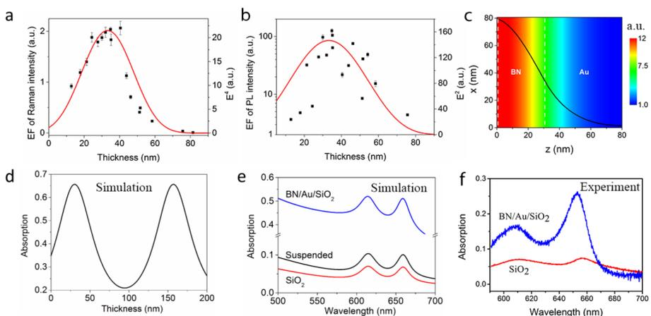
(a) Experimental EF of Raman  $E_{2g}^1$  peak intensity (black squares) and calculated  $E^4$  (red line). (b) Experimental EF of PL intensity (black squares) and  $E^2$  (red line). (c) Electric field intensity profile. (d) The calculated absorption of MoS<sub>2</sub> at 532 nm as a function of BN thickness. (e) (f) The calculated and experimental absorption spectra.
