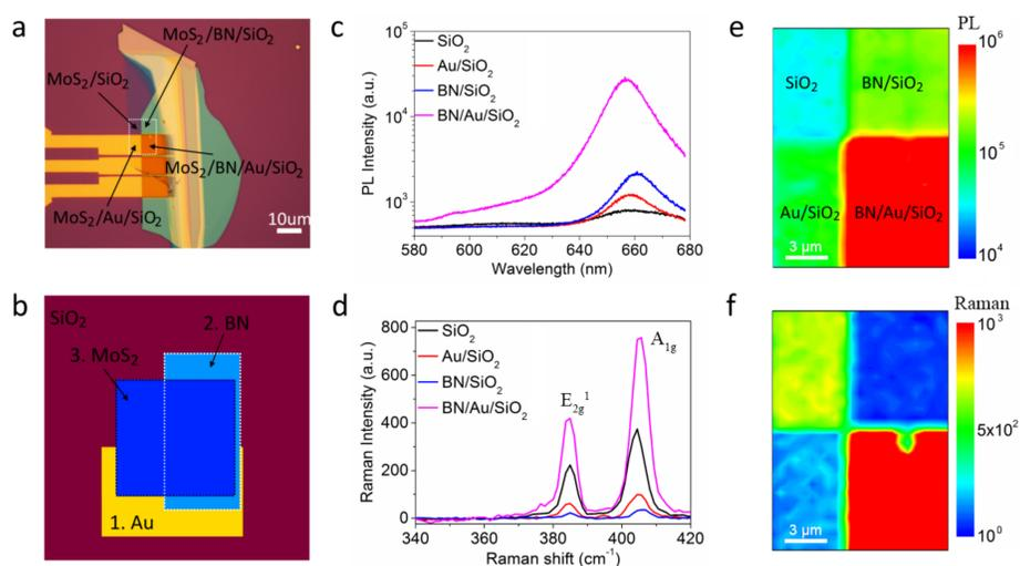
(a) Optical micrograph of monolayer MoS<sub>2</sub> on different substrates. (b) Schematic of sample preparation. (c) Semi-logarithmic PL spectra. (d) Raman spectra. (e), (f) PL and Raman mapping image respectively.
