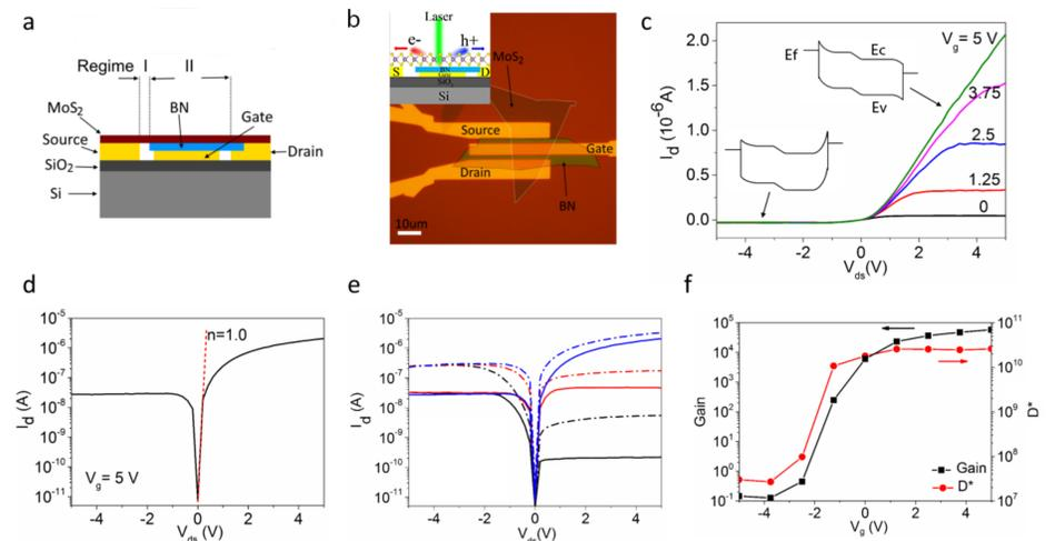
(a), (b) Schematic cross-section and optical micrograph of the device respectively. (c)  $I_d$ - $V_{ds}$  characteristics of the diode. (d) The ideality factor  $n=1.0$ . (e) Semi-logarithmic plots of  $I_d$  as a function of  $V_{ds}$  in dark (solid lines) and illumination (dash dotted lines). (f) The external photo gain (black squares) and specific detectivity (red dots).
