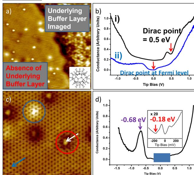
Fig. 2a) 20 x 20 nm STM image showing both quasi free-standing graphene and pre-existing graphene after intercalation. b) Averaged dI/dV spectra taken on i) pre-existing graphene and ii) decoupled graphene, indicated by a blue arrow. c) 7nm x 7 nm STM image of surface. d) dI/dV spectra taken over bright spots on decoupled graphene, as indicated by a white arrow.
