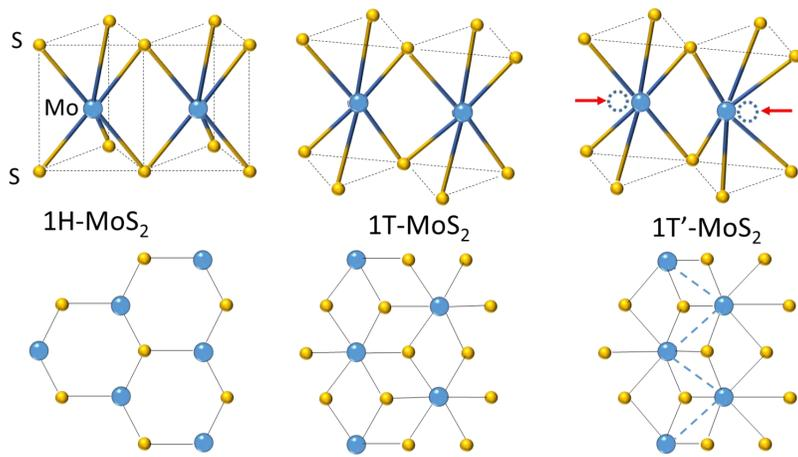
Three main phases that two-dimensional MoS<sub>2</sub> comprises. Trigonal semiconducting 1H-phase with a direct bandgap. Octahedral metallic 1T-phase which is reported to be unstable in free-standing conditions and will spontaneously relax to a distorted 1T' structure. Distorted transition metal atoms in the 1T'-phase form a period doubling 2x1 structure consisting 1D zigzag chains.
