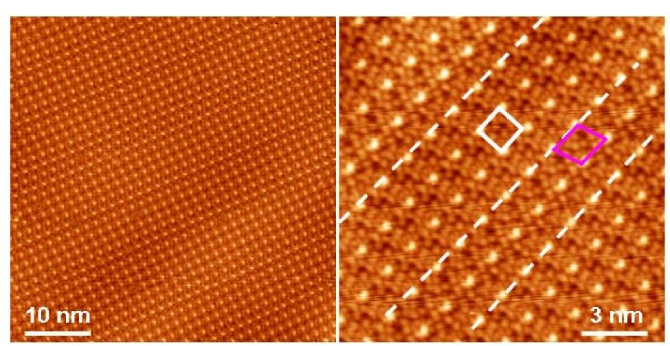
The disordered phase of ClAlPc on HOPG is composed of two different unit cells, as indicated by the white square and pink rhombic. Lattice mismatch between the neighboring molecular stripes is helpful for reducing intermolecular dipolar-dipolar interaction.
