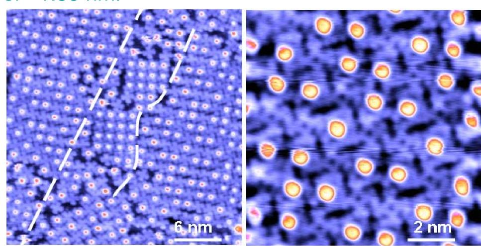
Monolayer CIAIPc on Au(111) with 60% molecules in CI-up configuration and 40% molecules in CI-down configuration. Regimes with short-range ordering are observed, formed by CI-up (CI-down) pairs alternating with CI-down (CI-up) single molecules.
