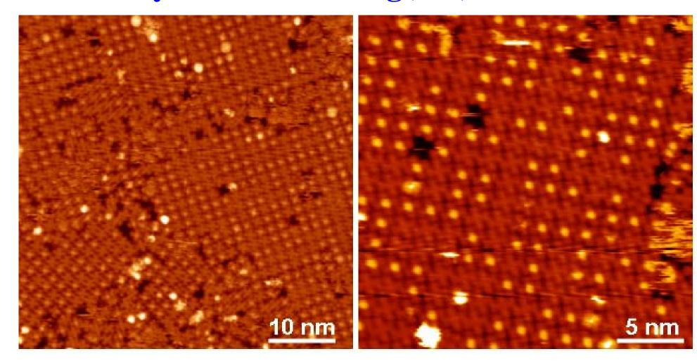
The monolayer CIAIPc on Ag(111) is composed of 50% CI-up molecules and 50% CI-down molecules. The distribution of the CI-up and CI-down molecules is disordered. It suggests that the interaction of the Ag(111) substrate with the CI atom is comparable to that with the molecular  $\pi$  plane.
