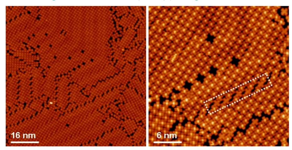
Monolayer CIAIPc on Au(111) after annealed at 200°C. The population of the CI-down molecules is reduced to 5%. Vacancies are also observable. The intermolecular distance is about 1.40 nm.
