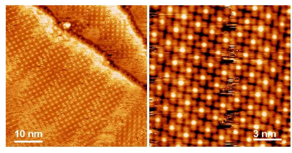
0.7 ML CIAIPc on Au(111) with Cl-up configuration. Loose-packing structure with intermolecular space of ~1.59 nm.
