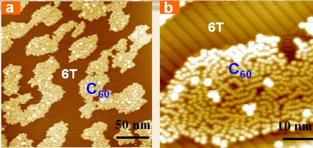
Figure 2 RT deposition of C<sub>60</sub> on 6T nanostructures: a, Large-scale image of 0.5ML C<sub>60</sub> deposited on 6T nanostructures at RT. C<sub>60</sub> molecules aggregate to form irregular shaped single-layer islands on 6T nanostructures. b, A detailed image indicates C<sub>60</sub> molecules form disordered worm-like structures.
