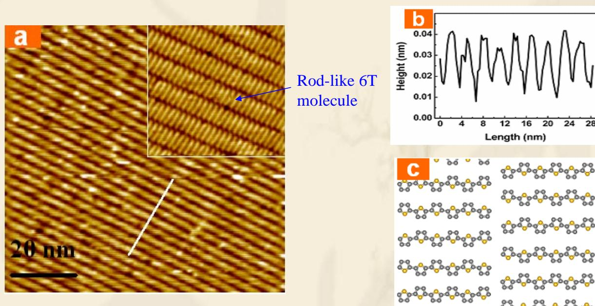
**Figure 1.**  $\alpha$ -sexithiophene (6T) nanostripes on Ag (111): **a**, STM image of the long-range ordered 6T nanostripes formed by annealing the Ag(111) covered with 1 ML RT deposited 6T at 400 K. Inset: a high resolution view of molecular structure on 6T nanostripes ( $I_t=150$  pA,  $V_{tip}=-1.70$  V); **b**, Cross-sectional profile along the diagonal white line in panel **a**; and **c**, Proposed model for 6T nanostripes on Ag(111).
