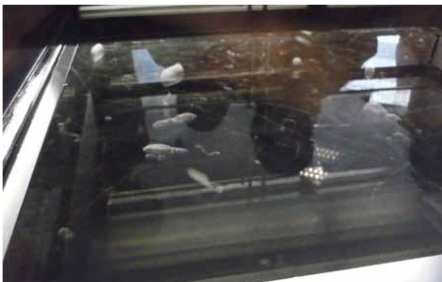
PhyWe cloud chamber: Thick tracks are due to alpha particles while thin streaks are due to beta particles.
