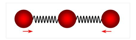
Eigenvector corresponding to  $\omega_2 = \sqrt{3}\omega_0 = \sqrt{3k/m}$ ,
