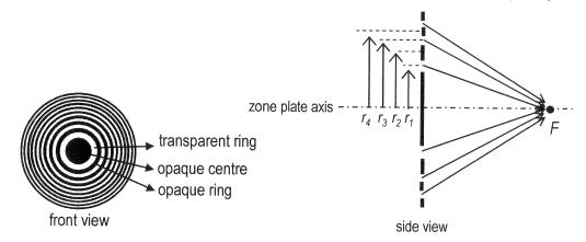
(i) Consider a wave passing through the transparent circular zone with radius  $r_m$  (where m is odd), and another wave passing straight through the centre of the zone plate if it were to be transparent. Write down the optical path difference  $\delta_m$  between the peripheral wave and this straight-through wave in terms of  $r_m$  and f. If  $\delta_m = \frac{m\lambda}{2}$ , show that this produces constructive interference at F, and so  $r_m$  is  $\frac{m^2\lambda^2}{2}$
