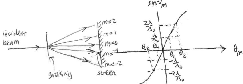
The  $m=0$  mode is the straight through mode. The positive and negative modes are symmetrically placed on each side of the  $m=0$  mode.
