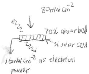
Assuming radiation is main heat loss mechanism,  $I_{rad} = I_{ex}$
