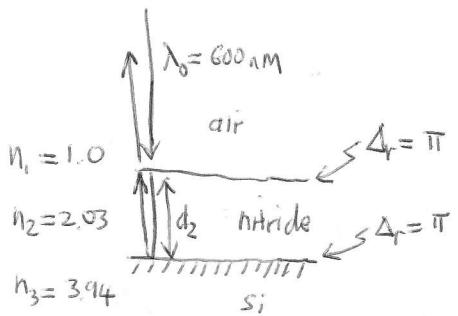
Since both  $\Delta_r = \pi$ , destructive interference occurs if the round-trip optical path in the nitride layer is a multiple of  $\frac{\lambda_0}{2}$ :
