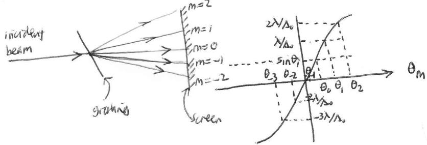
The  $m=0$  mode is still the straight through mode. The positive and negative modes are no longer symmetrically placed on each side of the  $m=0$  mode.
