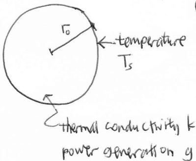
(i) At steady state, heat produced by sphere must equal heat convected at its surface.
