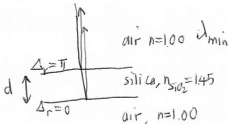
Constructive interference on reflection,
