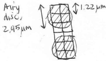
If a gap between two adjacent ink strokes is to be resolved, there needs to be a gap between the edges of the Airy discs. Assume a gap of 1 pixel, the centres of the Airy discs have to be separated by about  $2.5 + 1.0$  pixels = 3.5 pixels.
