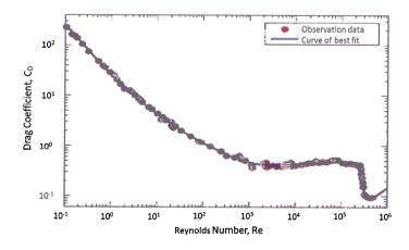
(a) Perform a dimensional analysis to derive the following expression for the drag D experienced by a sphere immersed in a steady flow of a viscous fluid:
