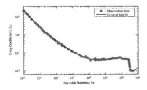
(a) Consider a viscous fluid of density  $\rho$  and viscosity  $\mu$  flowing around a sphere of radius a. The flow speed far from the sphere is U. Perform a dimensional analysis to show that the drag D experienced by the sphere is expected to depend on the various parameters in the following manner:
