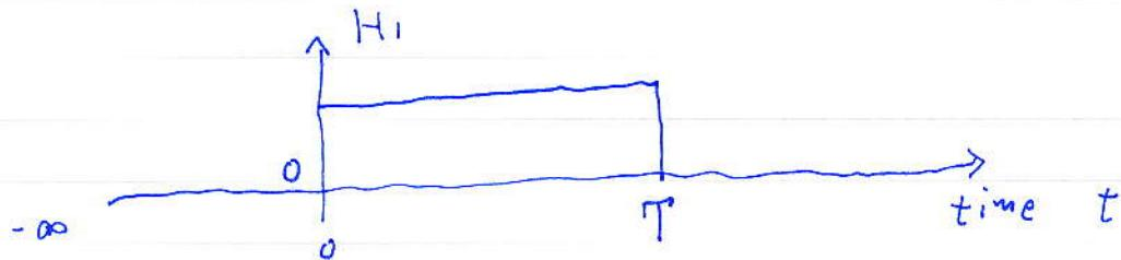
Due to the disturbance of  $\hat{H}_I(t)$  the system can not stay in the initial state  $|i\rangle$  but will make a transition to other states  $|i'\rangle$ . After  $t > T$  the transition stops and we are interested in the transition probability  $|\langle f | i \rangle|^2$ .
