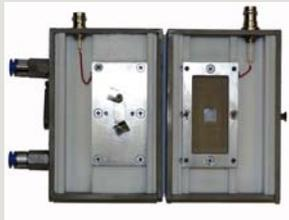
A graph showing the total-electron-yield detector consisting of two parts, a Cu mesh as anode and sample sitting on the aluminum plate, the outer shell is stainless steel
