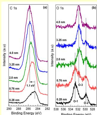
Fig.3 The evolution of (a) C 1s and (b) O 1s as a function of Alq<sub>3</sub> thickness on Co film. The C 1s and O 1s spectra were taken at photon energies of 350 eV and 650 eV, respectively.
