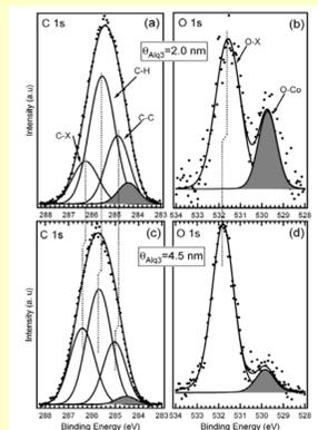
Fig.4 A fit to core level of C 1s (a), (c) and O 1s (b), (d) at normal thickness of 2.0 nm and 4.5 nm Alq<sub>3</sub>, respectively, for Alq<sub>3</sub> growth on Co thin film. Solid lines through the experimental data points demonstrate the results of least-squares fitting.
