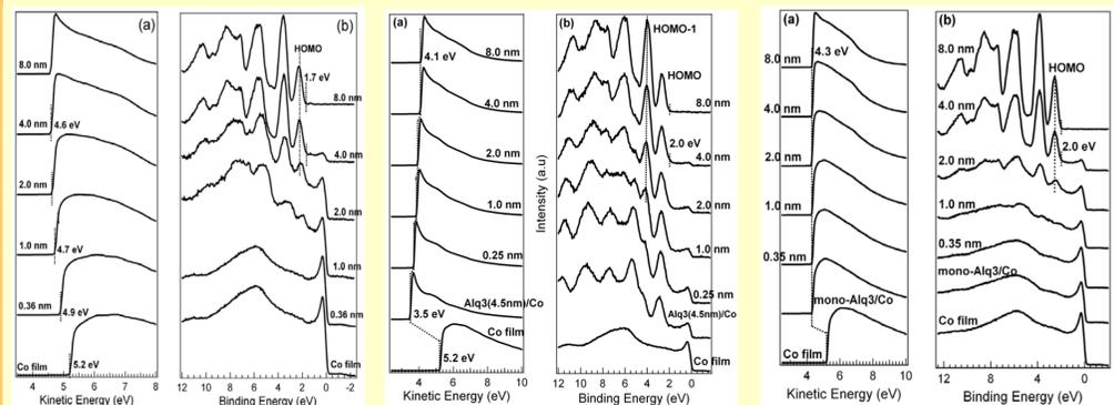
Fig.5 The evolution of (a) secondary electron cutoff and (b) valence band spectra as a function of C<sub>60</sub> thickness on Co substrate.
