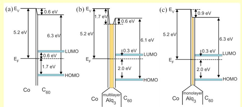
Fig.8 The energy level alignment diagrams for Co on (a) bare Co film, (b) multilayer Alq<sub>3</sub>/Co substrate and (c) monolayer Alq<sub>3</sub>/Co substrate.
